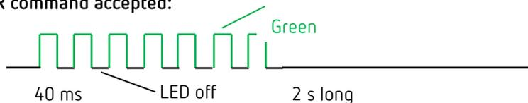
LED flickers (12.5 Hz) when a valid remote control command is received.
